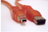
3. Plug into computer and to the camera's FireWire port.
